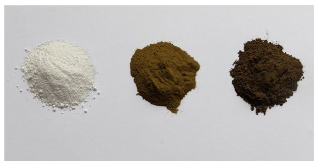
Image 1. Impurities in zinc oxide (ZnO) lead to significant differences in color and reactivity. Whereas pure ZnO is white (left), the presence of iron (middle, right) causes strong brown discoloration and hampers the reaction with acids, leading to lower ABC-4 values.
