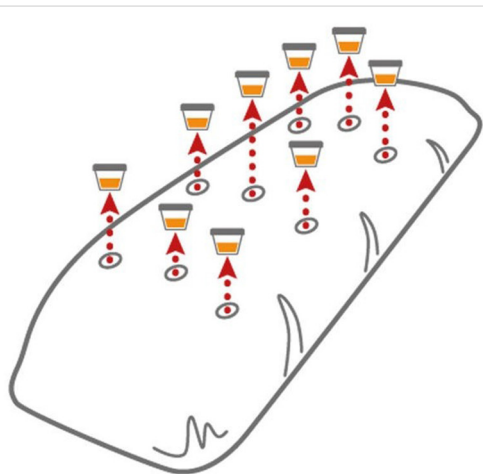
Figure 2. For bunker and bag silos, collect incremental samples by puncturing the plastic cover using a sharp, cone-shaped sampling device. Holes should be evenly distributed over the entire surface of the silo
